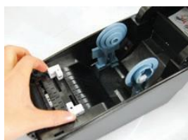
Transmissive sensor (Gap, Media sensor)
